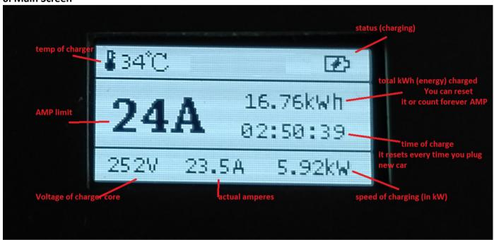
**Temperature of charger** – it is a temperature of core. It can be about 30-50C while charging and slightly more (like 60-65C) after disconnecting your car. This is normal, because fan cooling is stopped and core heat goes out by natural gravitational cooling.
