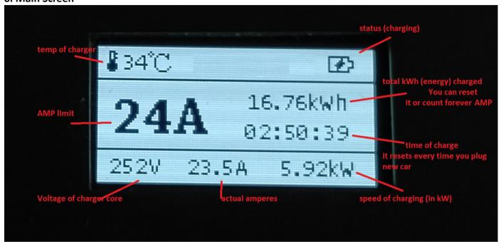
**Temperature of charger** – it is a temperature of core. It can be about 30-50C while charging and slightly more (like 60-65C) after disconnecting your car. This is normal, because fan cooling is stopped and core heat goes out by natural gravitational cooling.
